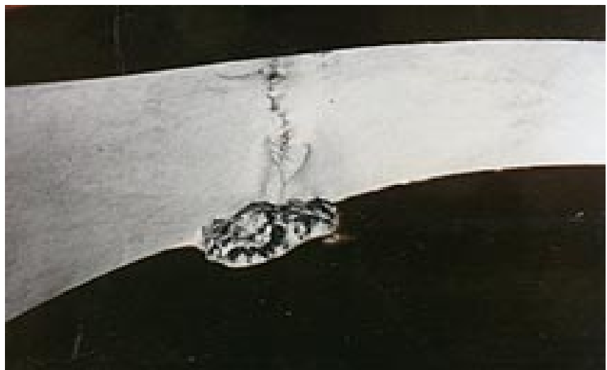
Figure 2 : Radial Puncture in Failed Bushing Porcelain
