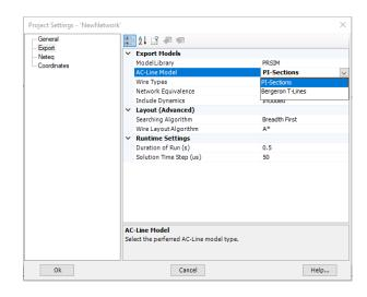
For IEEE14Bus system, selecting "PI-Sections" results in the following PSCAD case where all the transmission lines are represented by their PI section equivalent.
