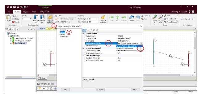
A pop-up window will provide access to Project Settings for the generated PRSIM case. By selecting "Export" and then "Network Equivalence", the user may choose to perform Network Equivalence from a dropdown list. Once "Perform Network Equivalence" option is marked, user may generate the PSCAD model by clicking on "Export Network". Network equivalent will appear as a module with a single or multiple ports representing the connection points to the rest of the system at boundary buses.
