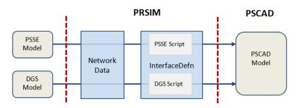
If the exported DGS file from PowerFactory or DYR file from PSSE contains any dynamic information, dynamic tables will be updated with such data during import process. To transfer dynamic information from relevant tables, user must include system dynamics in the export settings and finally click on "Convert Network". This option is automatically activated in presence of dynamic information.
