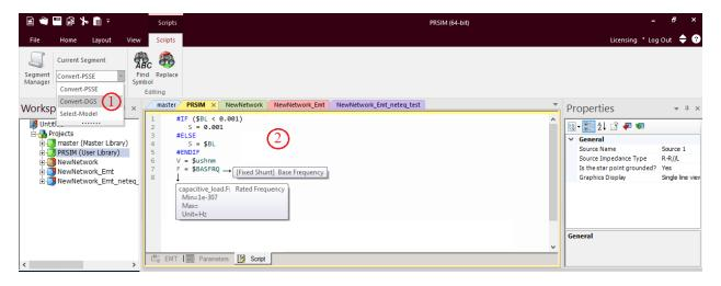
To add the script for conversion from DGS data, user must select "Convert-DGS" for Current Segment under "Scripts" tab and "Convert-PSSE" for PSSE part.
