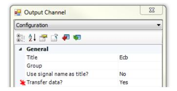
The ability to turn off data transfer will help to increase simulation speed when the curves obtained by a particular *Output Channel* are not required, without the need to delete the channel from the project.
